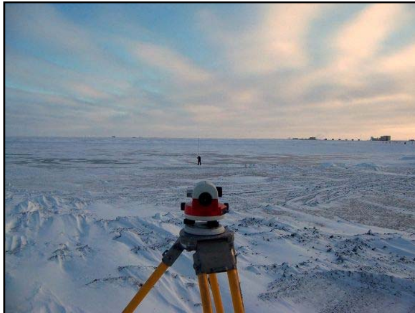
Figure 2. Surveying Water Surface Elevations at Kuparuk Deadarm Reservoirs, photo by D. Reichardt.
