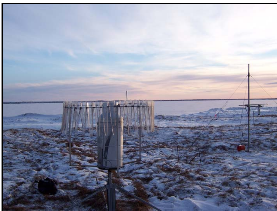
Figure 2. . Precipitation gauge at the L9312 weather station, photo by J. Derry.
