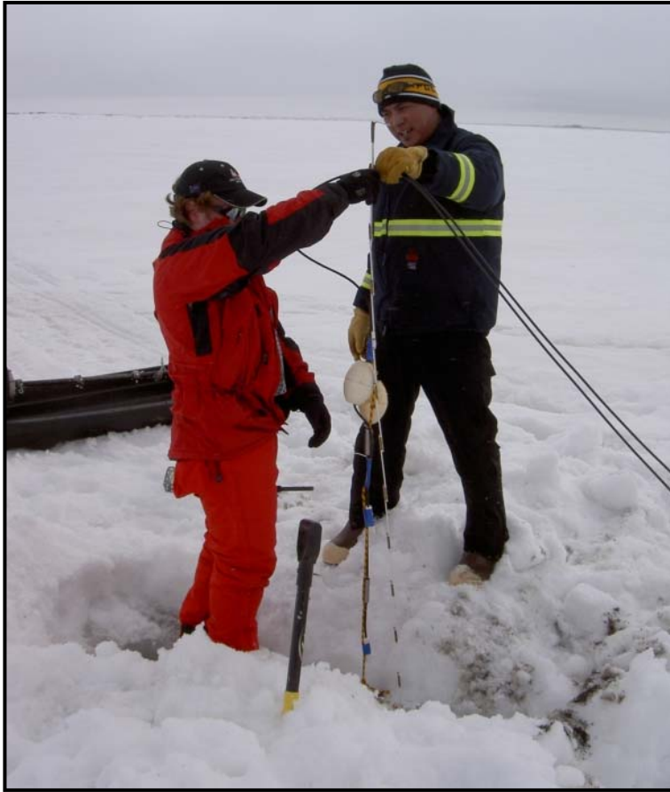
Figure 2. Inspecting deployed conductivity probe at L9312, photo by D. Reichardt.
