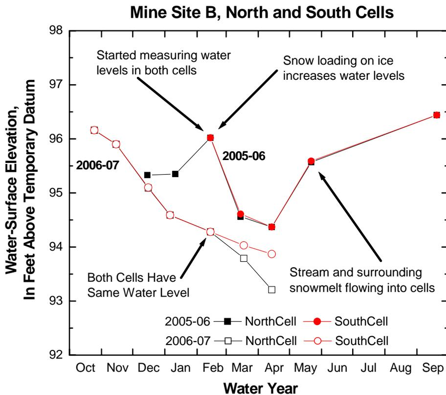
Figure 1. Water-surface elevation (temporary datum) in Mine Site B north and south cells. Data is shown for the 2005-06 and 2006-07 water years. The effects of increased water use can be seen in 2006-07.
