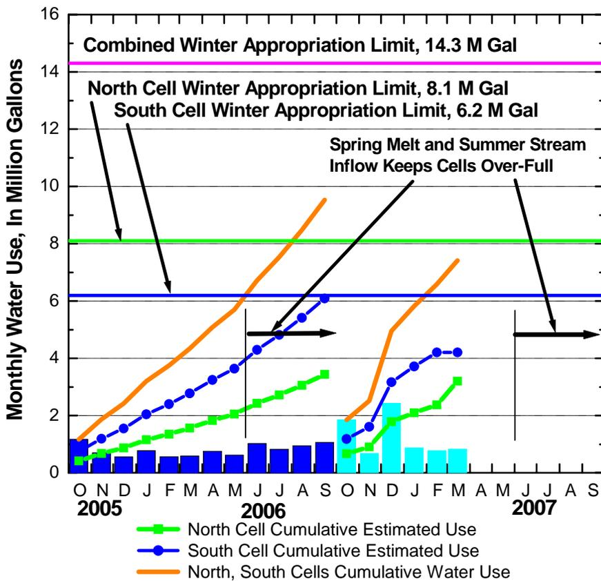
Figure 2. Monthly water use data for October 2005 through March 2007. Cumulative water use starts in October, coinciding with the water year and habitat permits. The combined water use is also shown for both cells, with separate and combined water use limits.
