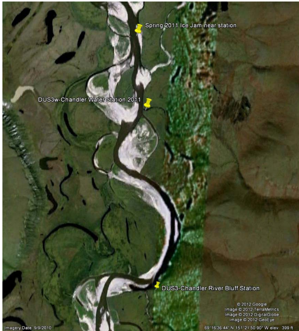
Figure 81. Location of old Chandler River observation station (DUS3) (which remains a meteorological station) on the bluff and the location of the new hydrologic station established in 2011 (DUS3w). An ice jam formed just downstream from the newly established station on May 22. Flow direction is from the bottom of the photo to the top of the photo (to the north).
