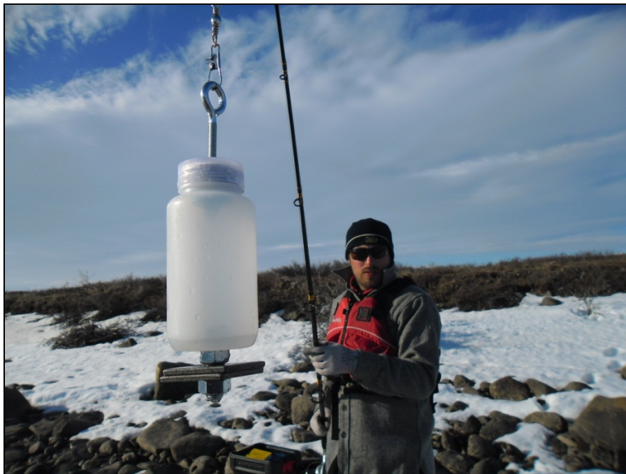
Figure 6. Sampling apparatus used to collect water samples at discrete intervals across the river.
