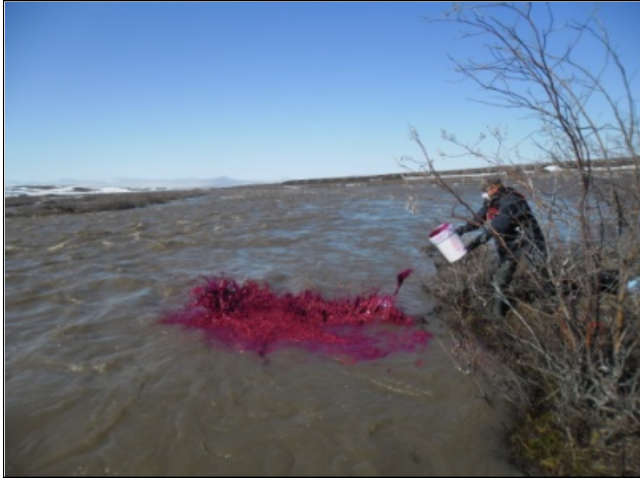
Figure 3. Researchers utilized the point slug injection method from a midstream gravel bar on May 25, 2011.
