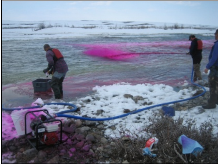
Figure 5. In two trials, a fire pump was utilized to distribute dye from the bank (May 20, 2011).
