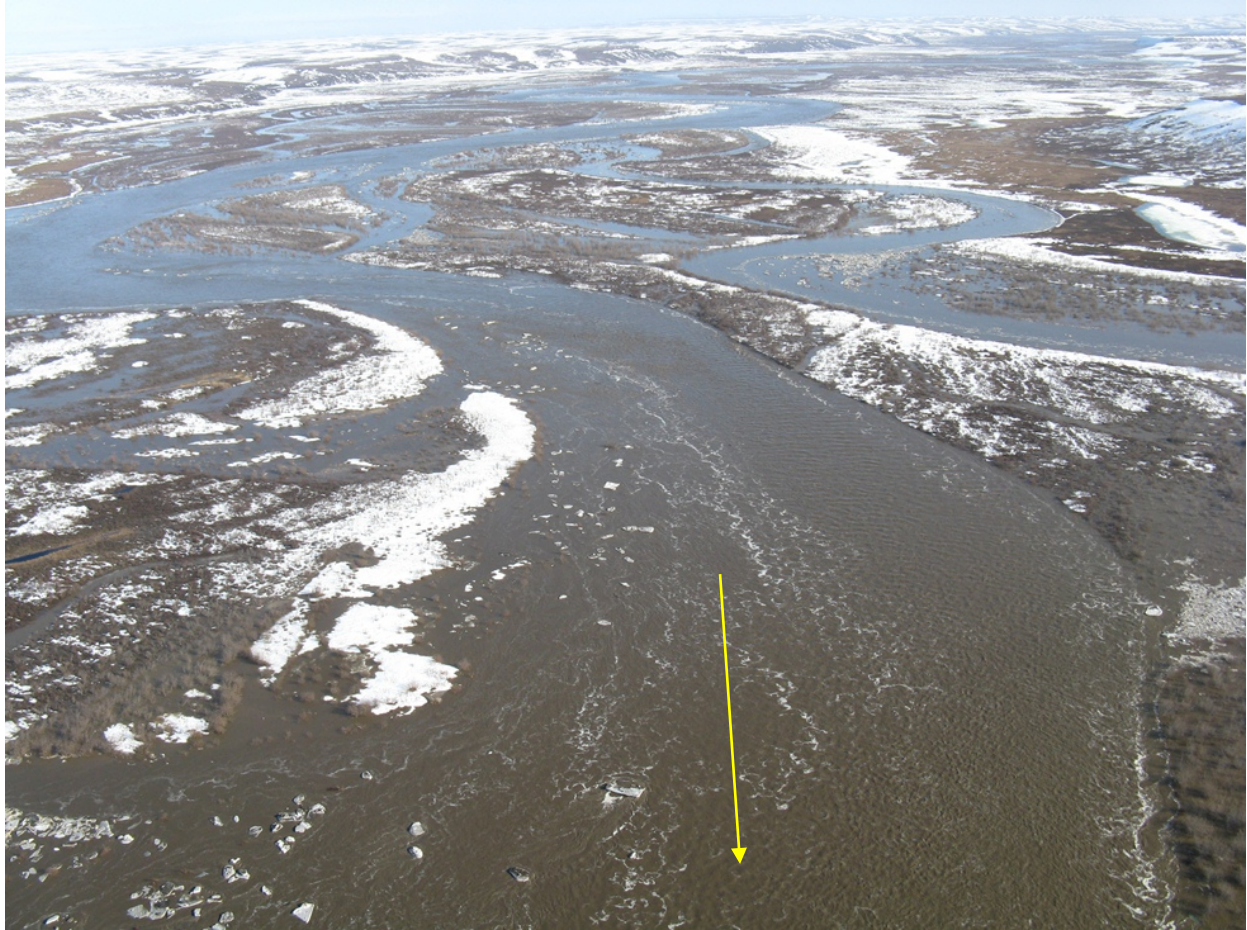
Figure 111. Chandler River on May 25, 2011, just south of the proposed bridge crossing (photograph taken toward the south) during the spring flood. Over-bank flow is visible, and significant flow occurs in side channels within the floodplain during very high stages.
