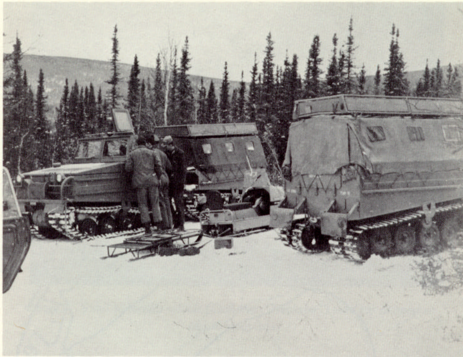
Figure 2. Low-ground-pressure tracked vehicle (Volvo BV-202A) used for off-road trail travel to field instrumentation sites.
