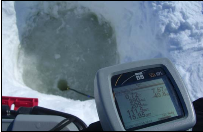
YSI Meter reading water quality parameters at Badami Pit, by Greta Myerchin.
