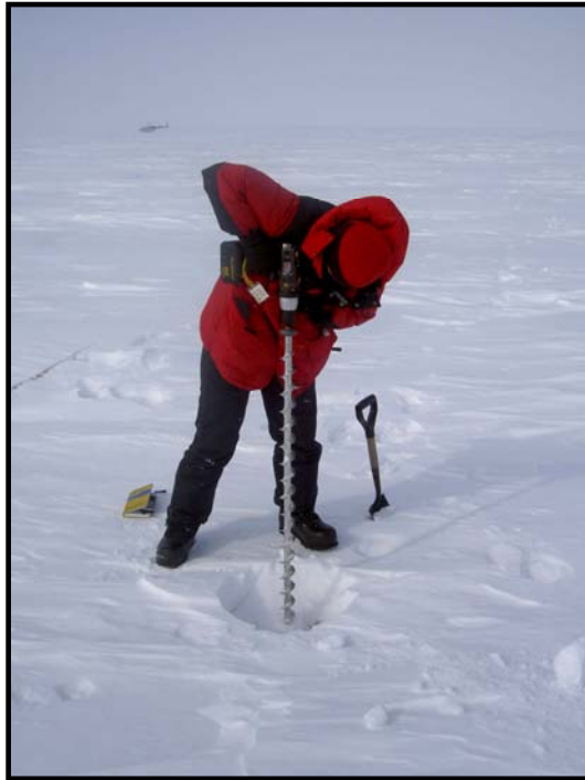
Drilling a sampling hole in lake ice, D. White
