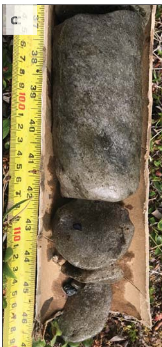
Figure A1.3 a. Borehole PLAY-1, elevation 3.1 m above sea level (a.s.l.), was drilled with the 3-inch diameter SIPRE corer in an ice-wedge trough. b-c. Photographs of the frozen core. At left ( b ), the protective intermediate layer of the upper permafrost (depth 76-93 cm) above the ice wedge is shown. Note inclined soil layers and ice lenses above the ice wedge ( b ) and gravel inclusions in wedge ice from ~105 cm ( c ). (Credit: M. Kanevskiy)
