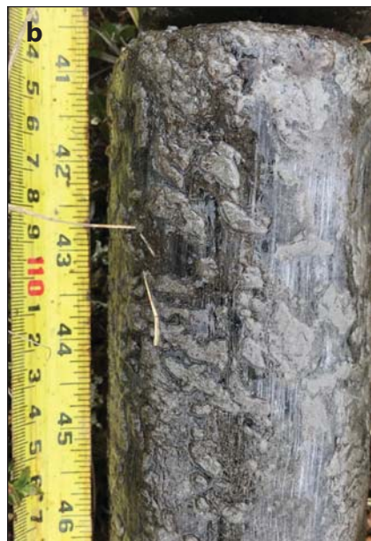
Figure A1.7. a. Borehole PLAY-10 was drilled with a SIPRE corer in a wet thaw lake basin with low-centered polygons, elevation 2.3 m a.s.l. b. Core shows ice-rich sandy silt with ataxitic cryostructure at depth of 104 to 117 cm. (Credit: M. Kanevskiy)
