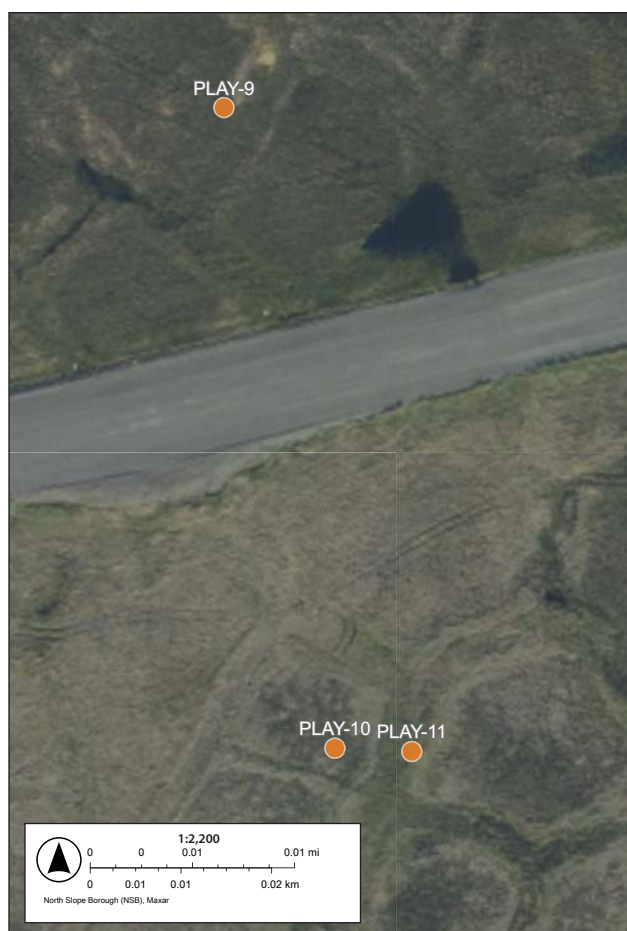
Figure A1.5. Boreholes PLAY-9 to 11 are in a large thaw lake basin along the Airport Road between the Airport Access Road and the Landfill Access Road. Borehole PLAY-9 and 10 were drilled from polygon centers. Borehole PLAY-11 was drilled from a thermokarst trough. All boreholes were drilled on 27 June 2022. (See Figure A1.1 for general location map.)
