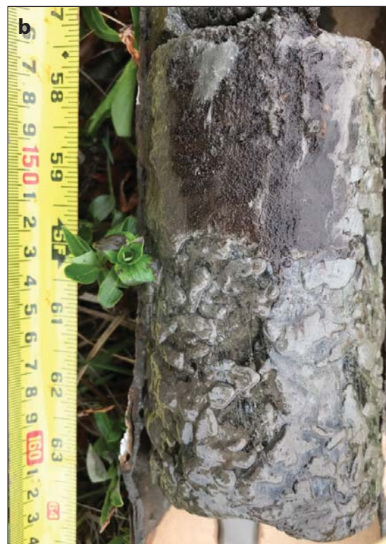
Figure A1.4 a. Borehole PLAY-3, elevation 9.2 m a.s.l., was drilled at the top of the baydzherakh (thermokarst mound). b. Analysis of the core at a depth of 147-161 cm shows an ice-rich sandy silt with vertically oriented peat inclusions and ataxitic cryostructure in silt. (Credit: M. Kanevskiy)
