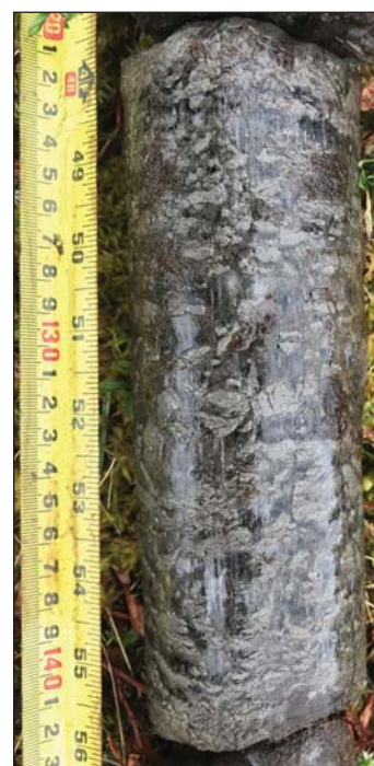
Figure A1.6. a. Borehole PLAY-9 was drilled with a SIPRE corer in a wet thaw lake basin, at 2.7 m a.s.l.. b. The permafrost core shows ice-rich sandy silt with ataxitic cryostructure from 122 to 141 cm beneath the surface. (Credit: M. Kanevskiy)
