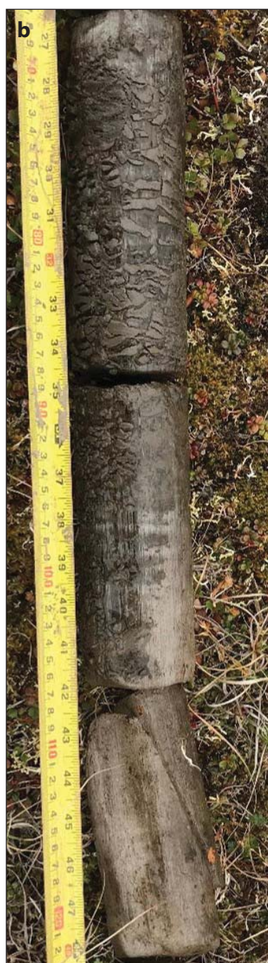
Figure A1.11. a. Borehole PLAY-26 at the center of a dry ice-wedge polygon, elevation 3.4 m a.s.l., was drilled with a SIPRE corer to 182 cm and with the Kovacs auger from 182 to 273 cm. b. The drilling analysis shows ice-rich silty sand from a depth of 68 cm and a buried ice wedge from 108 cm to 268 cm. (Credit: M. Kanevskiy)
