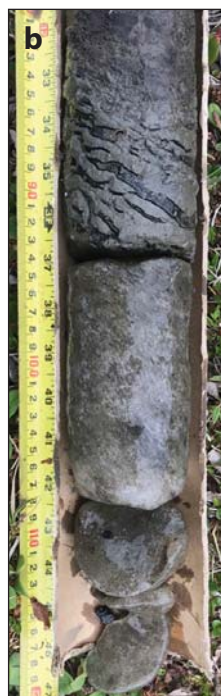
Figure A1.3 a. Borehole PLAY-1, elevation 3.1 m above sea level (a.s.l.), was drilled with the 3-inch diameter SIPRE corer in an ice-wedge trough. b-c. Photographs of the frozen core. At left ( b ), the protective intermediate layer of the upper permafrost (depth 76-93 cm) above the ice wedge is shown. Note inclined soil layers and ice lenses above the ice wedge ( b ) and gravel inclusions in wedge ice from ~105 cm ( c ). (Credit: M. Kanevskiy)
