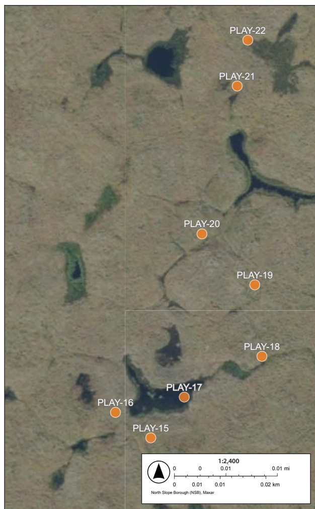
Figure A1.8. Boreholes PLAY-12 to 22 are located on yedoma terrain in the undeveloped area just north of the townsite townsite (boreholes PLAY-12 to PLAY-14 are not shown; they are located south of PLAY-15, see Figure A1.1 for general location map). Borehole PLAY-12 was drilled in a polygon center with a SIPRE corer to describe and sample frozen soils and ground ice. All other boreholes in this area were drilled in polygon troughs with a Kovacs auger to estimate the depth to wedge ice and vertical extent of ice wedges. All boreholes were drilled on 27 June 2022.
