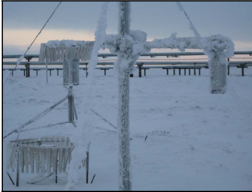
Figure 2. L9312 Meteorological station covered with rime and ice, Photo by J. Derry.
