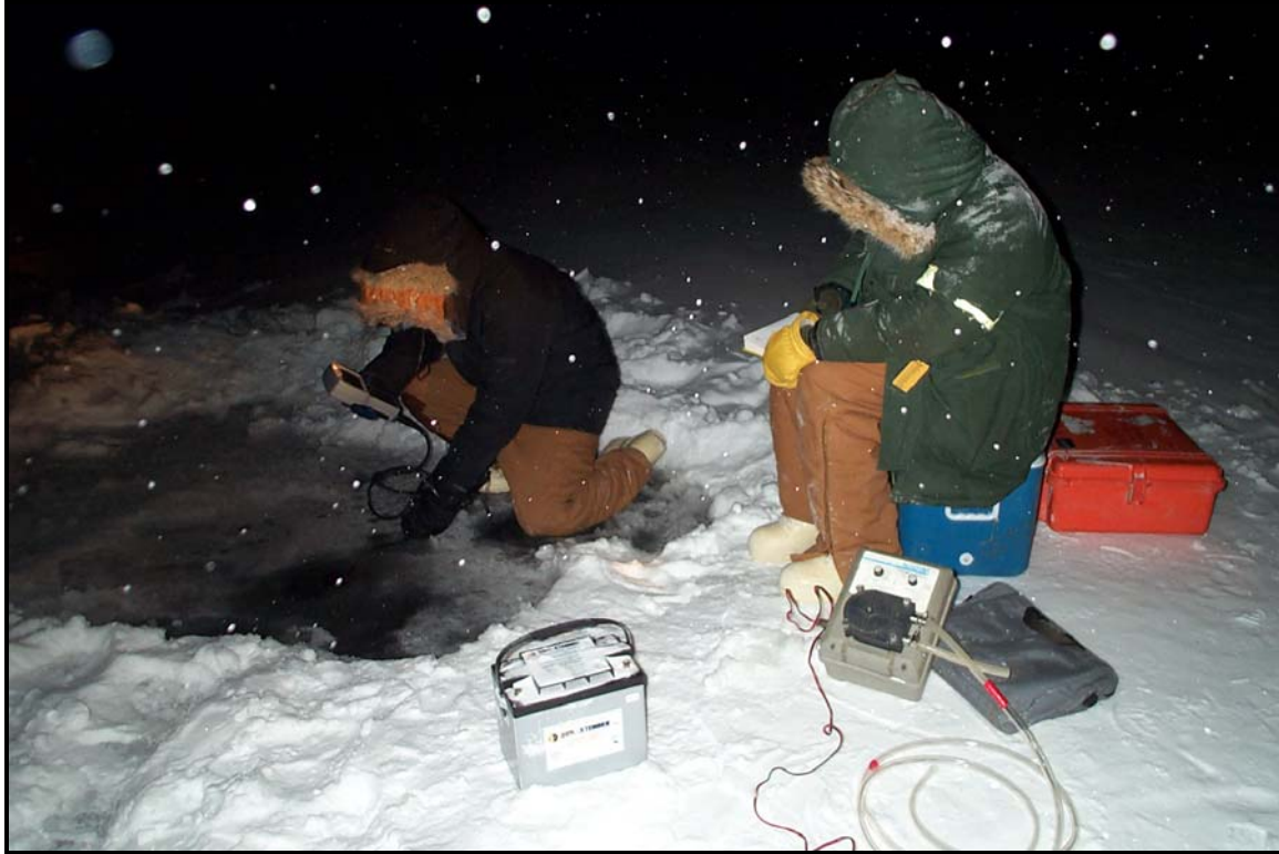
Figure 22. Both in-situ measurements of water characteristics (DO, conductivity, temperature, and pH) and water samples were collected at the lakes at several times throughout the winter.
