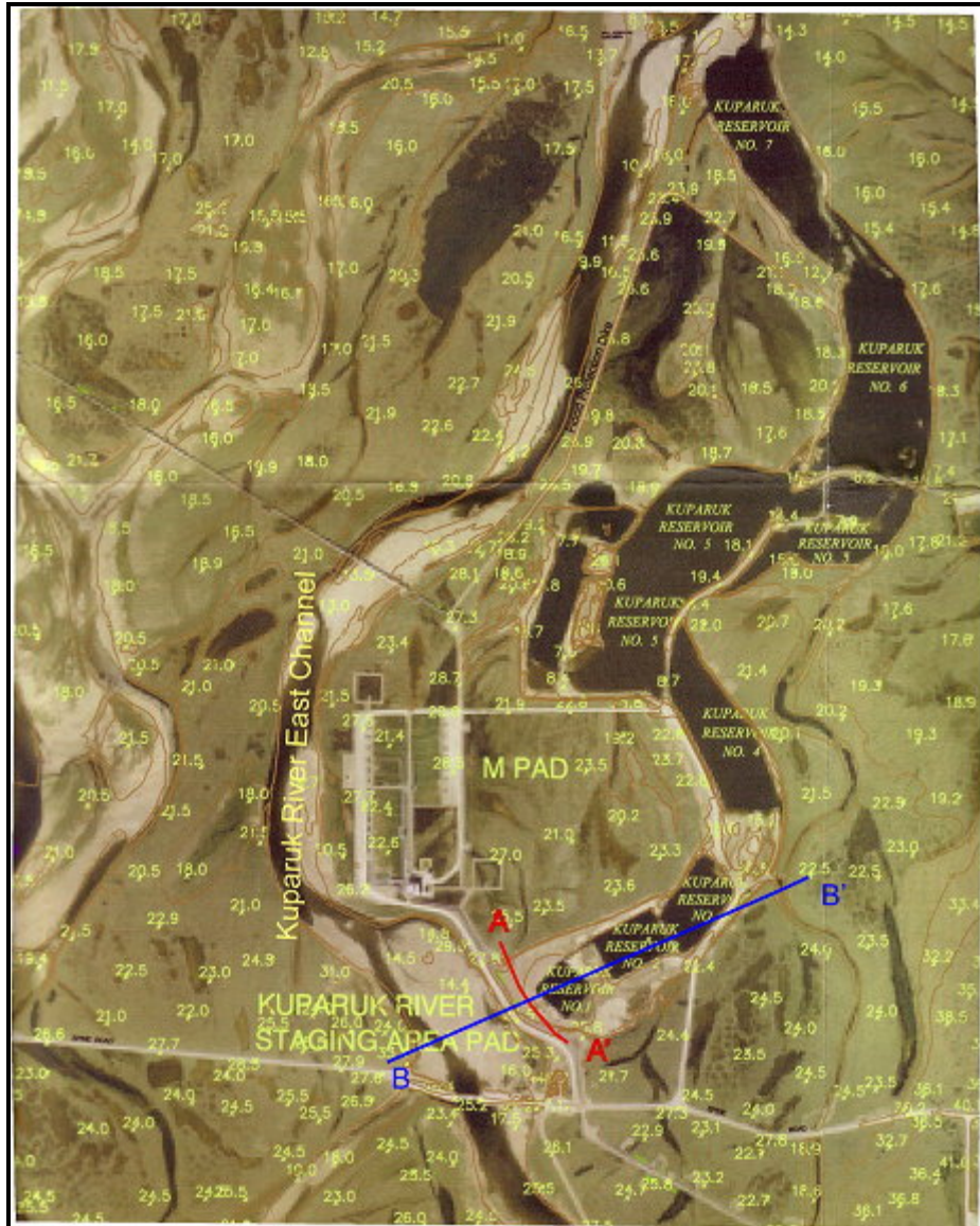
Figure 28. Study site and survey lines. Section B-B's also is used to help illustrate a hypothetical talik model for the area from the Kuparuk River east channel and cells 1, 2, 3 of the Kuparuk Deadarm Lakes.
