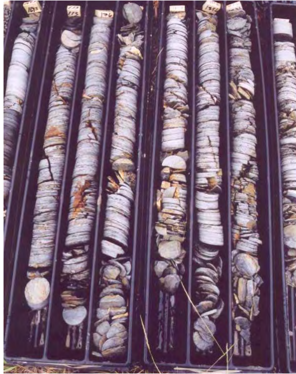
Figure 46: Core samples of the Birch Hill Sequence (photo by Emily Youcha, 2002).
