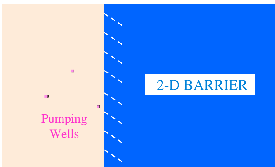
Figure 17. Plan view of Case 4 well vicinity. The low-K zone is shown as it is represented in WHPA.
