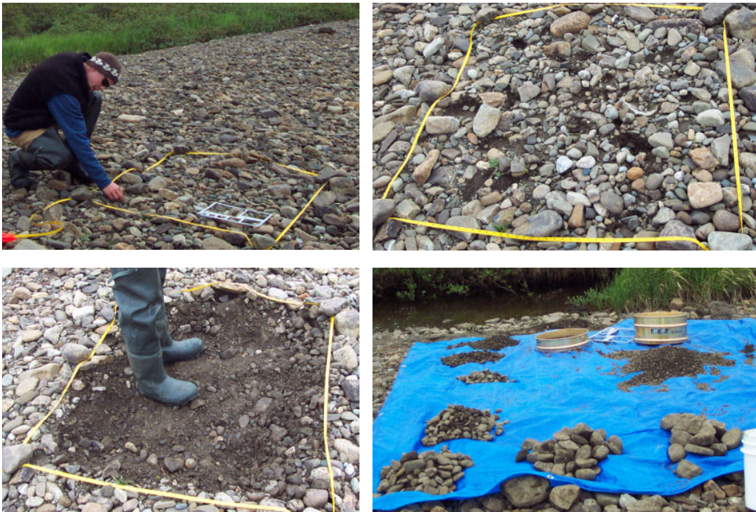
Figure 4.5 Subsurface pebble count. The area outlined (top left), surface pebble count performed (top right), material removed from area (bottom left), subsurface material sorted by size class (bottom right). (July 2002).
