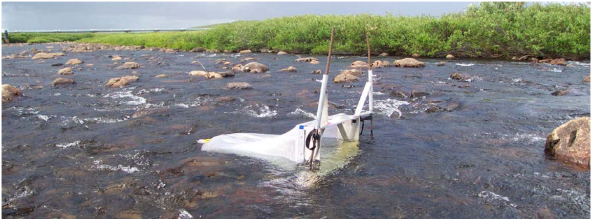
Figure 4.4 Bedload trap as installed in the Upper Kuparuk River (August 2001).
