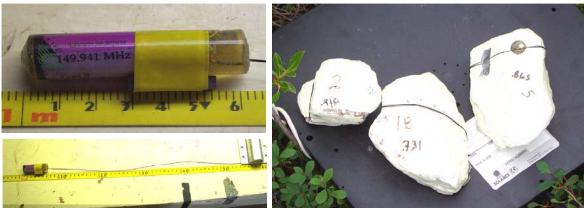
Figure 4.3 Radio transmitter used in active tracers (left top and bottom) and three active tracers prior to deployment (right) (July 2001).
