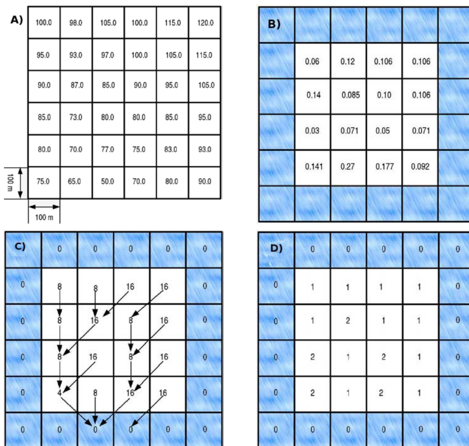
Figure 4.3. Digital Elevation Analysis. A) An example of a 100-meter DEM. Numerical values in each element represent the land surface elevation. B) The 'local slope' of each interior element. The 'local slope' is defined as the steepest (largest positive value) slope between an element and its eight neighboring elements. C) Flow routing. Each element is assigned a numerical value which designates the direction in which water from one element flows one of the adjacent eight elements. Arrows indicate direction of flow determined by the direction of the local slope. D) Order number. Each of these four files (DEM, Local Slope, Flow Direction, and Order Number) and an Information file must be generated prior to running TopoFlow. Note: Elements on the edge of the DEM (shaded elements) are not considered part of the model domain.
