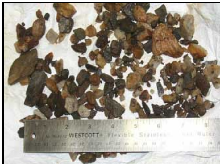
Figure 6. Photograph of valley bottom gravels (photograph by Jim Vohden). Ruler shows units of inches on top.
