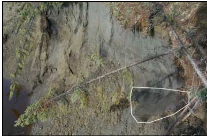
Figure 7. Photograph of Fairbanks Silt and ice lens (outlined in white) at the Yellow Eagle 99Pit (by Jim Vohden).
