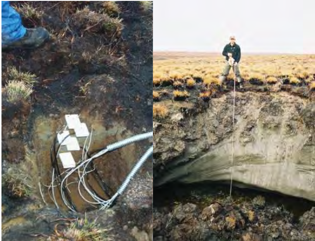
Figure 2.5 K2 soil moisture sensors were re-installed in October 2002 at 5, 10, 15, 20 and 30 cm depth. The photo shows the fire severity through the reduced organic material between the tussocks. Right: Erosion of Niagara Creek with exposed ice-rich permafrost in September 2003. The gully has become wider and longer since then, reaching 275 m in length by fall 2006. Substantial ground subsidence has occurred along the banks, resulting in more gentle sides. Note that the tussocks survived the fire.
