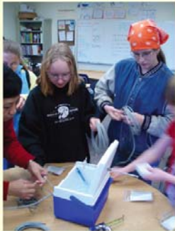
Sensor calibration sensors are calibrated in ice bath (0°C) (Healy, AK)
