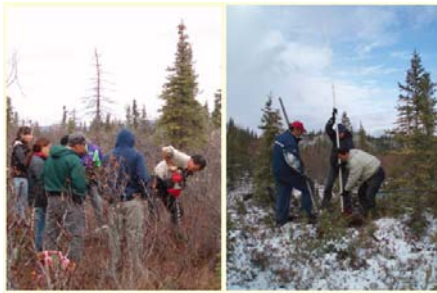
Drilling: takes most time and effort. The depth of the borehole may depend on the underlying soil type. (Noatak, AK)
