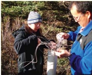
Sensor installation sensors are lowered down the borehole and the cables carefully connected to the datalogger (Healy, AK)
